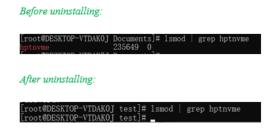
e. If the system does not display information about "**rsnvme or hptnvme**", the driver has been successfully uninstalled.
