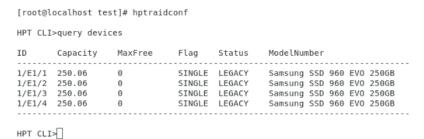
5. If the WebGUI/CLI can connect to the controller and recognized the NVMe SSD's, the driver has been installed and is functioning normally:
